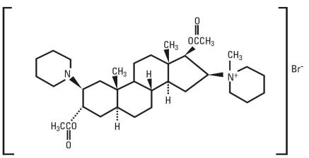
Its chemical formula is  $C_{34}H_{57}BrN_2O_4$  with molecular weight 637.73.
