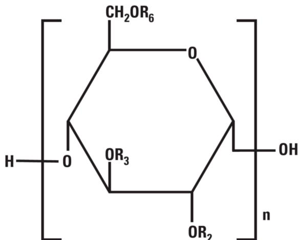
Amylopectin derivative in which  $R_2$  and  $R_3$  are H or  $CH_2CH_2OH$  and  $R_6$  is H,  $CH_2CH_2OH$ , or a branching point in the starch polymer connected through an  $\alpha$ -1,6 link to additional D-glucopyranosyl units
